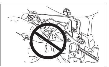
Figure 22. Linkage and Lever Bending
